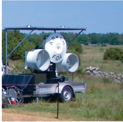
Figure 25: The FOI Arken radar [111]. The left antenna is used for transmission and the right for reception. The middle antenna is used for special purposes. The radar is pulsed and can operate in 6-18 GHz for both horizontal and vertical polarization. This radar is used in [23, 105]. Photo by FOI.
