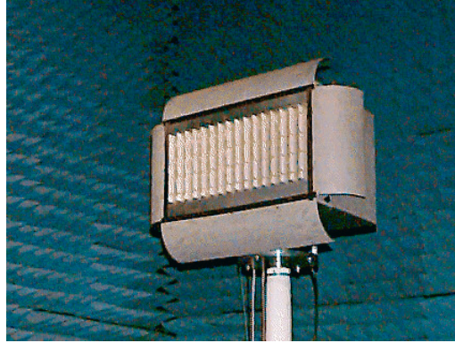
Figure 13: The FOI DigAnt receiving array antenna [59, 60] in an anechoic chamber. The digital array is linear in the horizontal direction with 12 digital channels. It was designed and built by FOA (FOI) and Ericsson Microwave Systems (Saab Electronic Defence Systems). This antenna is used in Publication 1 (reference [3]), 2 (reference [4]) and 4 (reference [6]) and in [27, 28, 29, 59, 60, 61, 62, 63, 64]. Photo by FOI.
