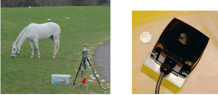
Figure 27: Left: The IMST radar and a radar target. In the micro-Doppler mode the radar is a pure-carrier radar with frequency 24 GHz and vertical polarization. The radar antenna and RF electronics, which are manufactured by the German company IMST, are mounted on top of the tripod. The box on the ground contains the control computer. Photo by Karl-Göran Stenborg. Modified by Svante Björklund. Right: Close-up of the IMST radar antenna and RF electronics module. Photo by Svante Björklund. This radar is used in Publication 9 (reference [11]).
