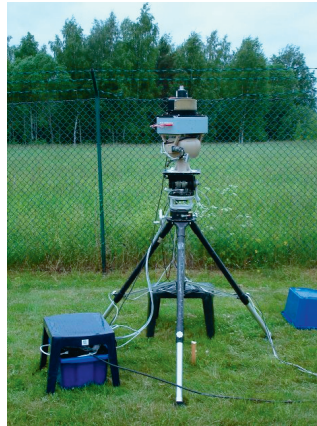
Figure 26: The Saab SIRS 77 radar. It is a single-channel pulsed FMCW (Frequency Modulated Continuous Wave) radar operating at 77 GHz with horizontal polarization. It has a resolution in range of 1 m and in azimuth of 1^\circ . The radar antenna, RF electronics and a turn table are mounted on top of the tripod. This radar was used in Publication 8 (reference [10]) and in [12, 16, 18, 112, 113]. Photographer: Svante Björklund. Photo from [17]. Reproduced with permission from DGON (German Institute of Navigation).
