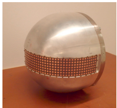
Figure 16: Experimental conformal antennas on a half-cylinder (diameter 30 cm) for 16-18 GHz, designed and built by FOI. Both antennas have 35 \times 7 antenna elements. Left: Planar facets. Photo from [66]. Also present in [7, 19]. Right: Smoothly bent aperture. Photo Svante Björklund.
