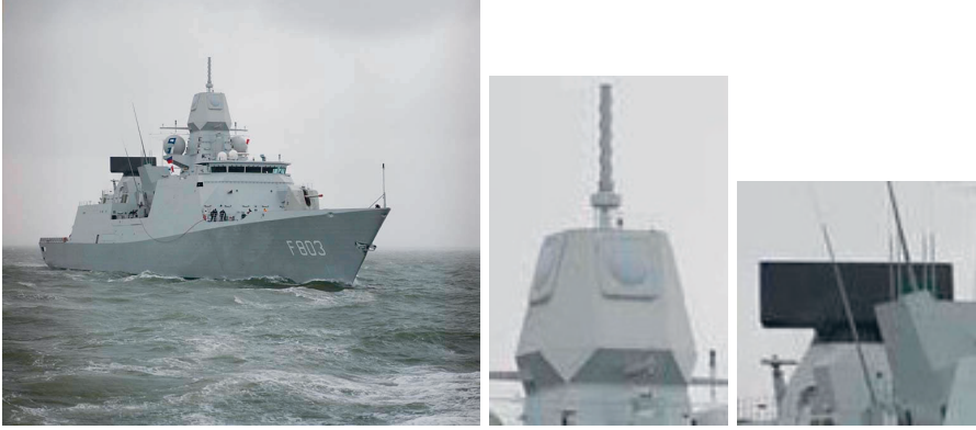
Figure 9: Left: The frigate HNLMS Tromp (F803) of the Royal Netherlands Navy with the APAR and the SMART-L radars. Middle: The APAR Naval radar with two of the four fixed planar antenna apertures visible. Right: The SMART-L radar. The rotating antenna is the dark rectangle. It is a vertically steerable array. All three photos: Royal Netherlands Navy / Koninklijke Marine [50].
